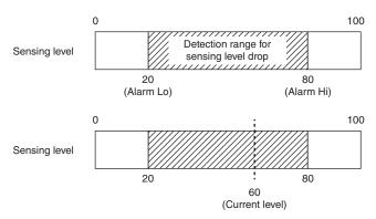
If this condition continues for 5000ms (equipment parameter 5:  $50 \times 100$ ms), it is detected as a drop in the sensing level and the user is notified with the ALM indicator on the unit and the alarm information is sent to the status detail area\* on the master unit.
