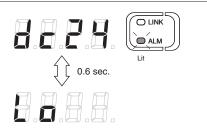
If the voltage of 24V DC power supplied to the unit becomes significantly low (near 16V), the message "dc24 Lo" is displayed and the unit stops functioning. Check the supply voltage and take actions to increase the voltage to the allowable range.
