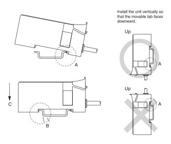
Push the unit in the direction of D and free the fixed tab B from the DIN rail. While keeping the unit pushed, pull it up in the direction of E to lift the body and take it off the rail.
